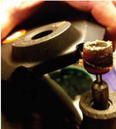
Grind small amounts and keep checking to see the fitment
